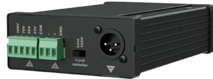
The ATU44MK2 is a universal input adapter unit for conversion between various audio level signals, offering a wide variety of connection and extension possibilities to audio systems. The speaker level input features various taps for 100V, 70V, 50V and 33V audio levels, while a balanced line input allows conversion between balanced and/or unbalanced line level audio signals.
