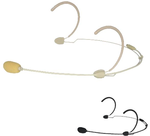
The CMX826 is a headset condenser microphone with a directional cardioid pick-up pattern, designed for professional 'hands free' voice reinforcement or recording applications. The cardioid pick-up pattern guarantees an excellent rejection of background noise and feedback, allowing it to be used in acoustical demanding applications or situations where the performer is positioned in front of loudspeakers or monitors.
