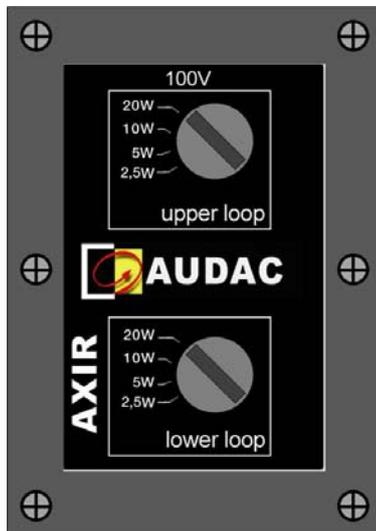
To reach the internal switches, the plate with the two power tap selector switches should be removed. This can be done by loosening the 6 Phillips screws whereby it is attached.
